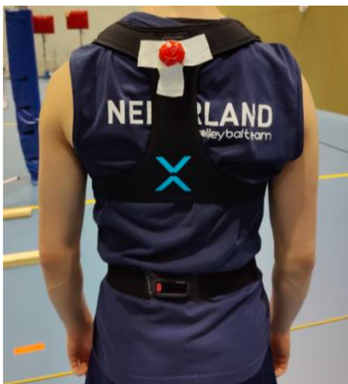
Figure 1. Participant wearing the Kinexon harness (with red semi sphere attached over the sensor) and Vert elastic band
