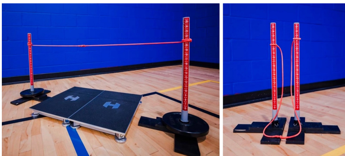
Figure 2. Modified range of motion (ROM) monitoring setup and bilateral force plates by Hawkin Dynamics™, USA.
